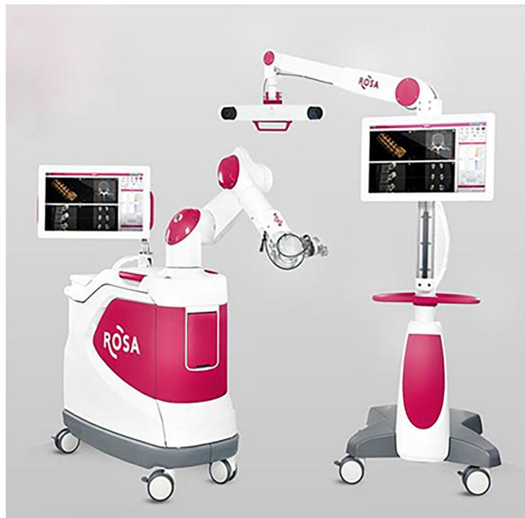
**Figure 1** Rosa spine robot platform. Freely mobile floor-mounted base station with arm (left) and optical infrared tracking camera (right).
